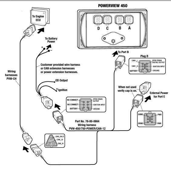
\* Note: Ignition must be connected to the battery or to an ignition switch for the display to turn "ON".
