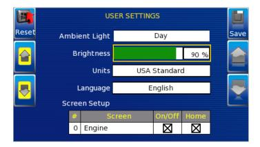
**NOTE**: Brightness level will change with ambient light setting. Two brightness levels are saved; one for day and one for night.
