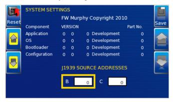
The yellow **Up** and **Down** keys on the left allow you to move the cursor through 'J1939 Source Addresses' fields. While the cursor is highlighting a field, the gray **Up** and **Down** keys scroll through available options. Once all the options have been selected, press **Save**.
