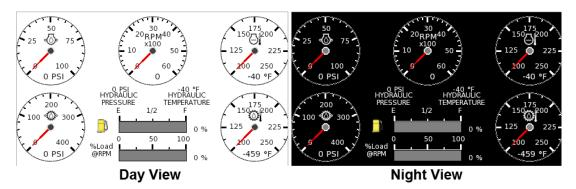
**NOTE:** The ambient lighting option is also accessible through soft key commands on the gauge display screens. When selected, the **Day/Night** soft key toggles the display to the opposite mode.
