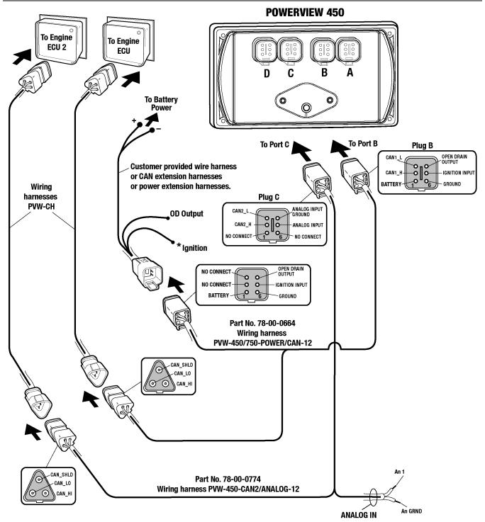
**NOTE:** Port B and C connectors are keyed differently than Port A and D connectors to ensure proper connection.
