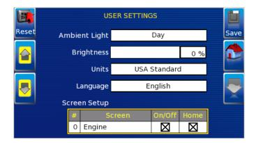
The Screen Setup screen also provides the user the ability to turn the screens ON or OFF by pressing the **Enable/Disable** soft key. If a screen is turned OFF, it will not show up when Gauge Display is activated.
